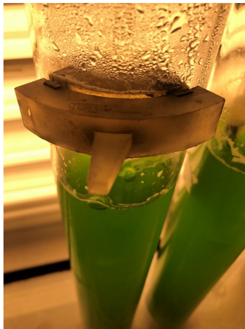
Figure C.4. 3-D printed algae scrubbers that was to resuspend the biomass that was lost back into the medium.
