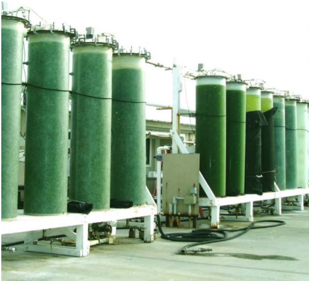
Figure 2.4. 400-liter column closed culture system used in Cyanotech Corporation during the astaxanthin production from H. pluvialis ( http://www.cyanotech.com/ ).
