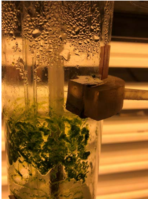
Figure C.3. Problem seen with the tube reactors ( e.g. biomass loss).
