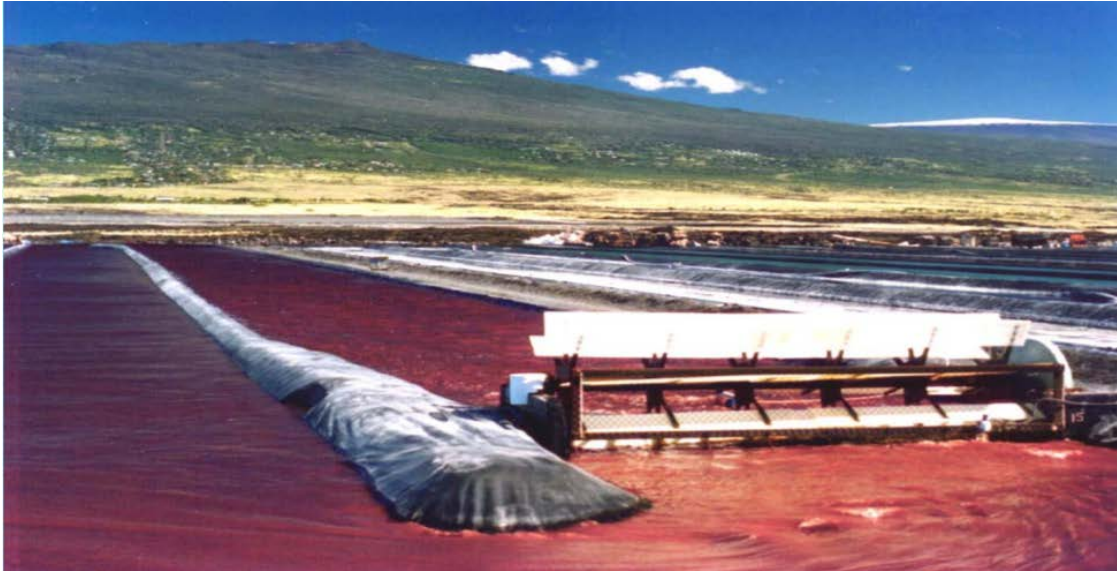
Figure 2.5. Final stage of astaxanthin production from H. pluvialis carried out in Cyanotech Corporation. 500,000-liter open system ponds ( http://www.cyanotech.com/ ).
