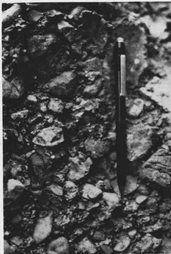
Figure 13. Close-up of crudely stratified conglomerate (Gm/Dcm) from upper member showing poorly-sorted and muddy nature of matrix.
