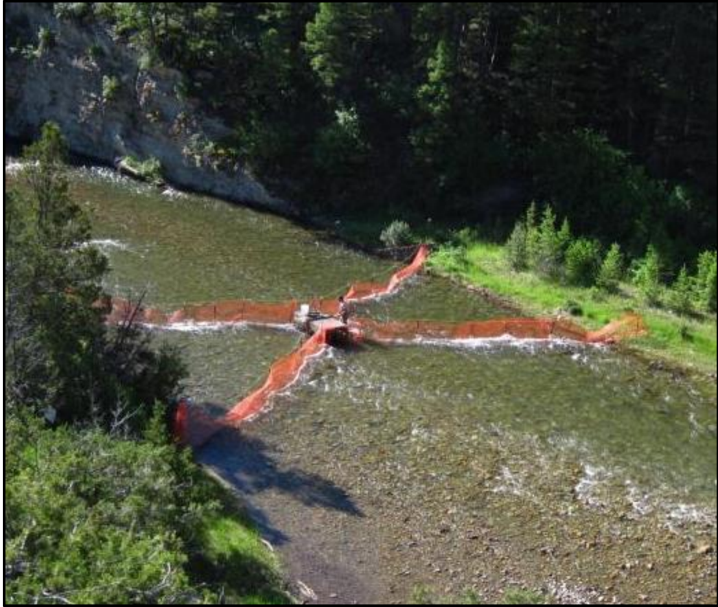
Figure 11. The upstream and downstream fish weir operated about 350 m upstream of the confluence of Tenderfoot Creek with the Smith River. The weir was operated 4-7 days every month from July to October in 2011 and 2012.
