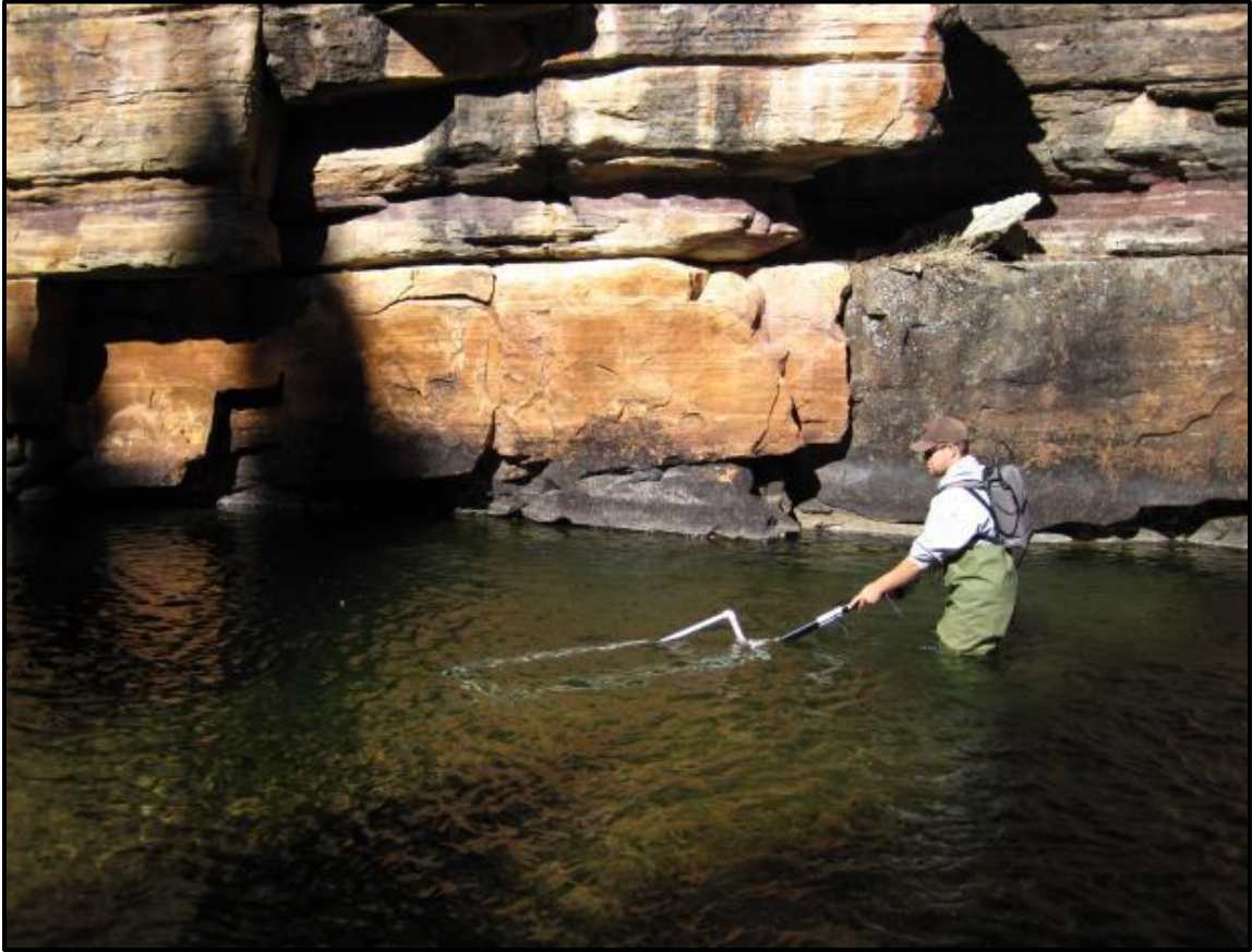
Figure 14. Wading antenna being used during a portable antenna survey in Tenderfoot Creek in October of 2011.
