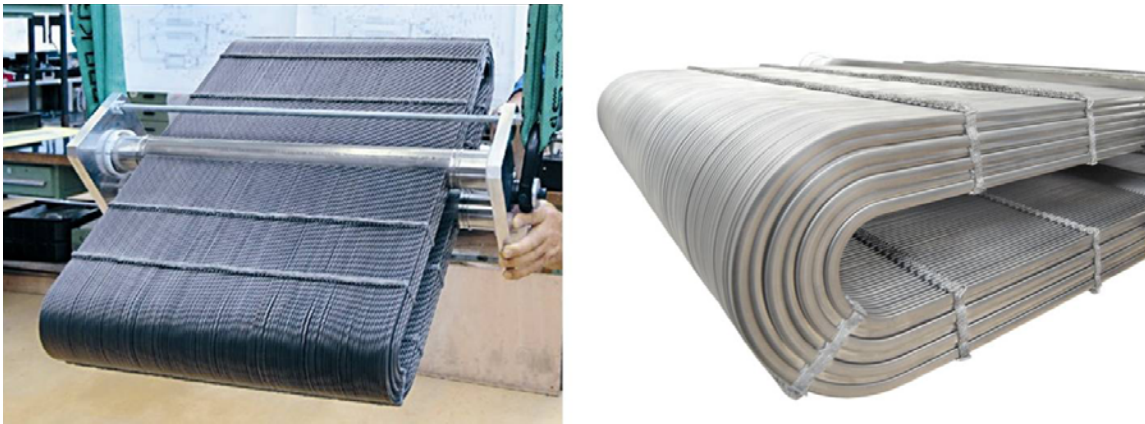
Fig. 6. Recent Fin-Tube Design (permission to use this image was granted by MTU Aero Engines GmbH, see Appendix A)
