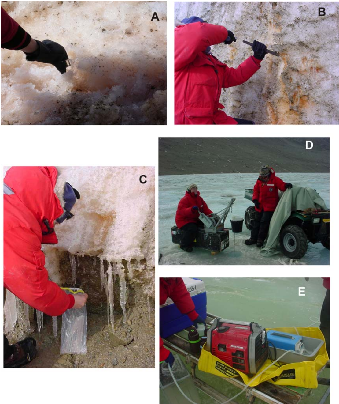
Figure A.9. Diverse modes of sample collection at Blood Falls. When primitive flow was active, samples were collected directly into sterile containers (A), ice was chipped with sterile tools (B) or removed as icicles (C). When outflow occurred below the ice, the ice was drilled and samples were collected with a Niskin bottle (D). Slow, ponding outflow was collected with a peristaltic pump and tubing (E).
