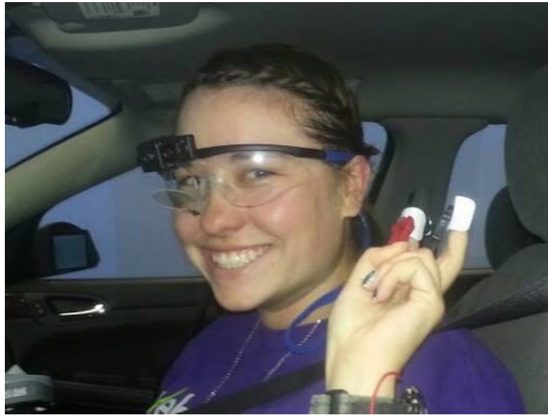
Figure 10. Participant wearing ASL eye tracker with EDA leads in place.
