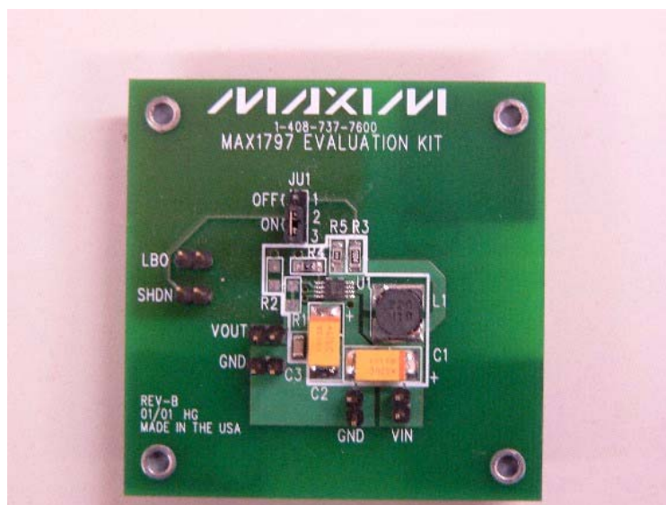
Figure 2.5. Max1797evkit DC-DC converter used to power the temperature sensor.
