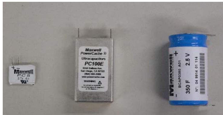
Figure 2.4. Ultracapacitors from left to right: 4 farad, 100 farad and 350 farad
