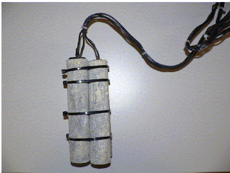
Figure 2.3. Four sacrificial magnesium anodes bound together with a tie-strap.
