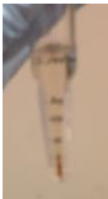
Figure 5.2. Ni-NTA and Q-sepharose purification of XcbA2 yields pinkish or when more concentrated, a reddish-brown enzyme. The picture depicts a 30 kDa molecular weight cutoff filter that appears to have concentrated XcbA2 towards the bottom of the cone, indicating that the color is a feature of the protein and not an artifact of the cell lysate.
