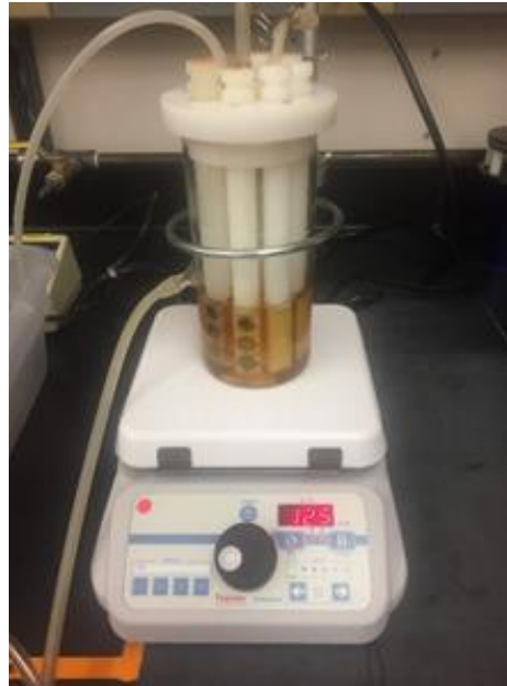
Figure 2.1: CDC biofilm reactor containing E. coli K12 biofilm growing on aluminum and silicon nitride substrate samples.
