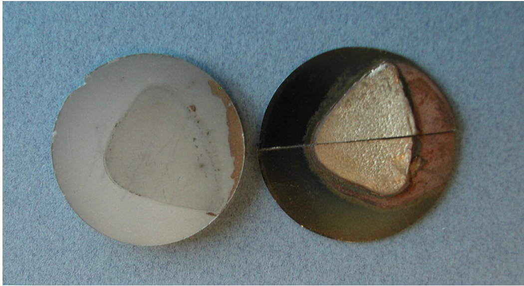
Figure 37 MSU1H Vacuum Braze Joint
