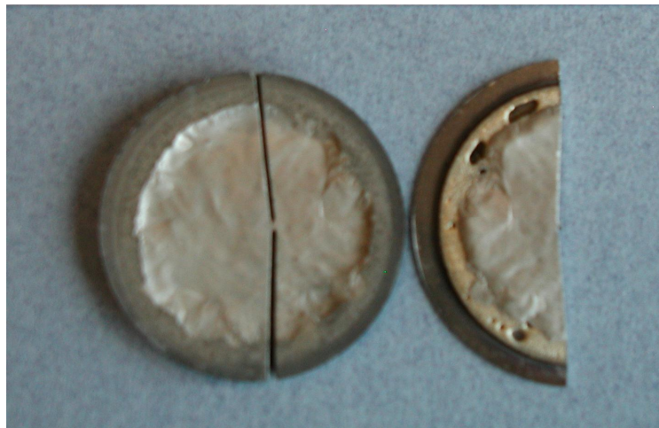
Figure 49 Fracture Pattern of MSU3 Argon Braze Joint
