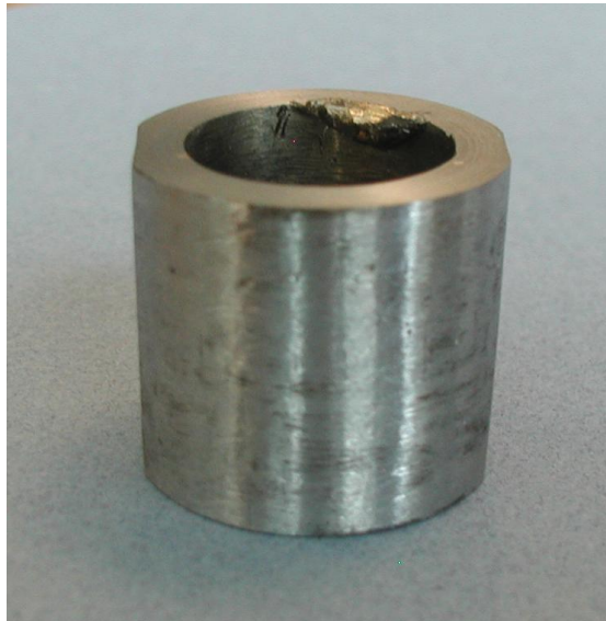
Figure 16 440 Stainless Steel Machined Rupture Cup
