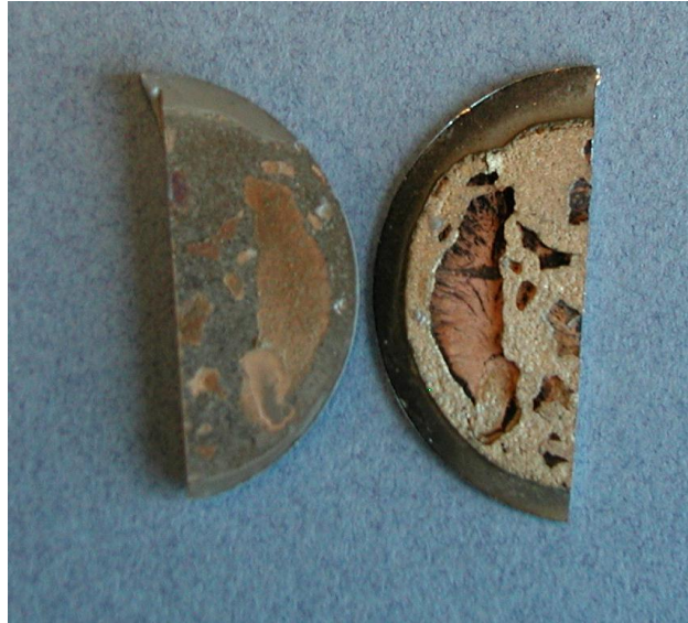
Figure 45 MSU6 Vacuum Braze Joint
