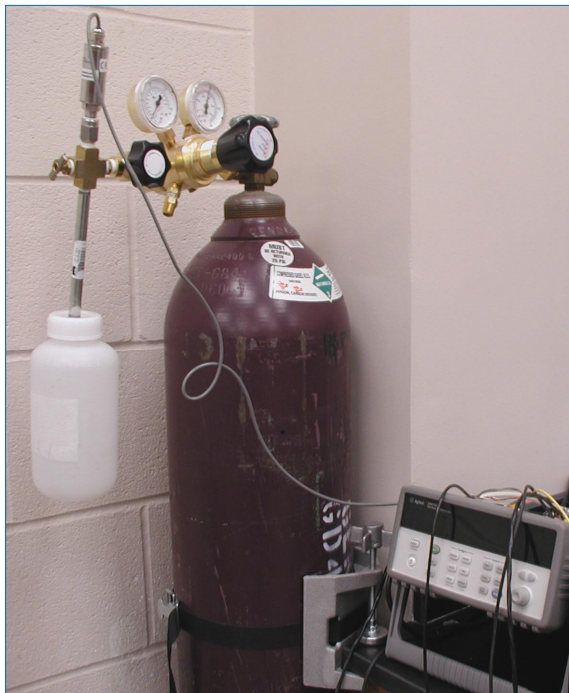
Figure 17 Experimental Set-up for Pressurized Rupture Test
