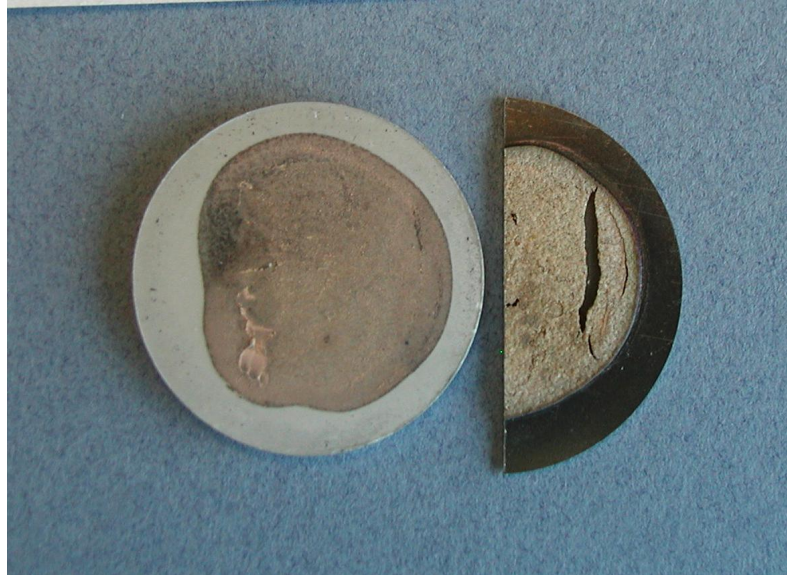
Figure 41 MSU2 Vacuum Braze Joint
