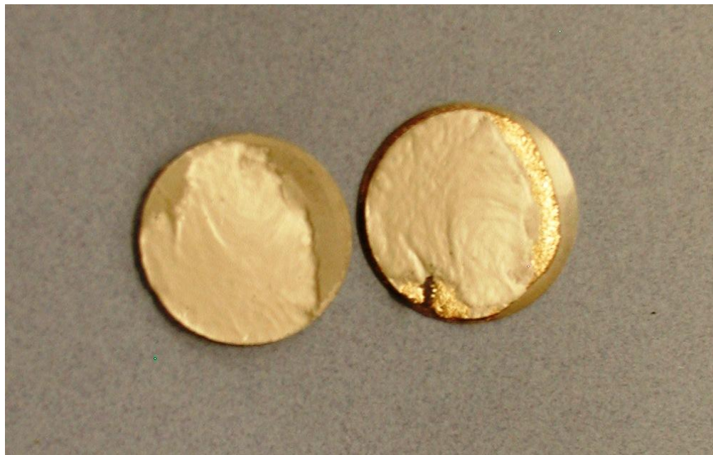
Figure 60 Fracture Pattern for MSU3 In-House with the Addition of ALT
