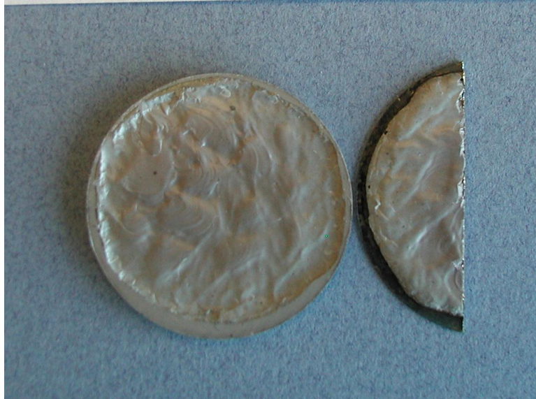
Figure 42 MSU3 Vacuum Braze Joint
