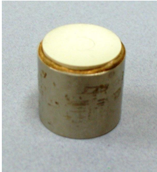
Figure 29 Rupture Test Sample for Copper ABA Vacuum Braze
