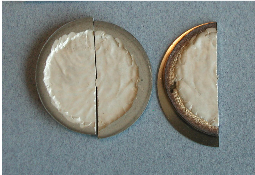
Figure 27 Fracture Pattern of Copper ABA Argon Braze Joint
