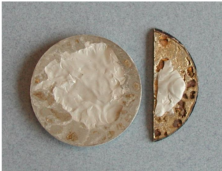
Figure 54 Fracture Pattern for MSU3 Atomized Alloy
