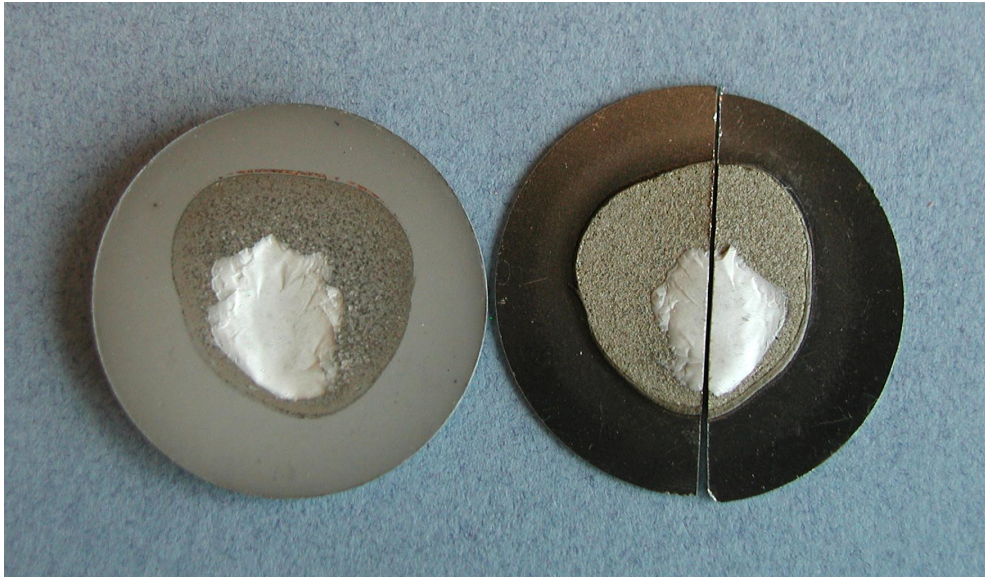
Figure 44 MSU5 Vacuum Braze Joint
