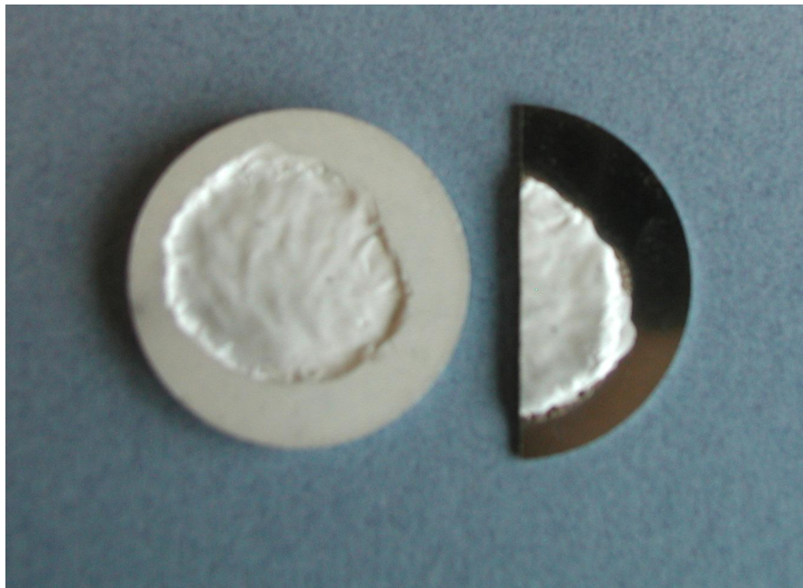
Figure 21 Copper ABA Vacuum Braze Joint
