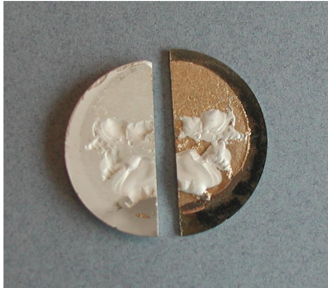
Figure 38 MSU1 Vacuum Braze Joint
