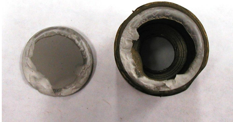
Figure 50 Pressurized Rupture Test Cup for MSU3 Alloy Brazed in Vacuum
