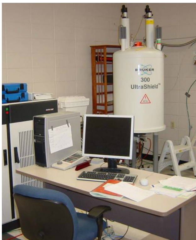
Figure 1.11. The 250 MHz superconducting magnet used for experiments in this thesis
