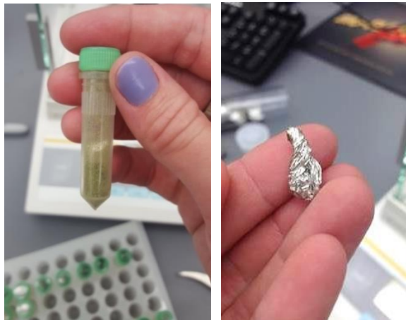
Figure 2.4: Left: Dried whitebark pine needles ground in screw cap tubes. Right: A sample packaged in a tin capsule.
