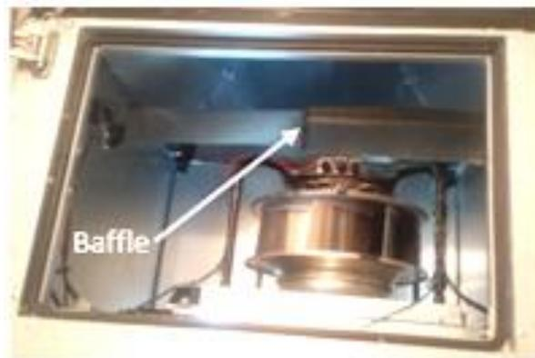
Figure 3.4: Wing baffle location
