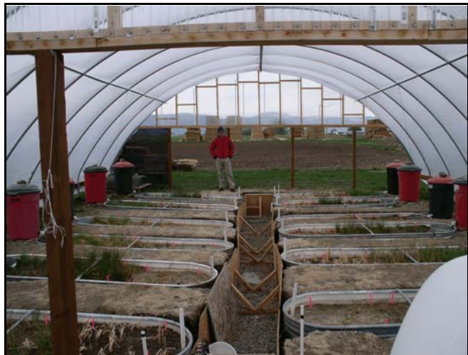
Figure 6. Installed and planted lysimeters.
