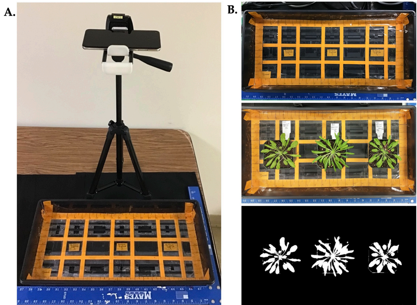
Fig 1. Image station setup for Canopeo imaging under lab environment. (A) A tripod is set up at 64 cm (25 inches) height to take images using cellphone with Canopeo app. Tripod feet were centered behind the tray, using the square ruler as a guide for repeatable placement. (B) A dark colored background was used as an imaging backdrop. A dark colored tray with gridlines was used for the repeatable spacing of specimens. Digital images were uploaded to the Canopeo app using the smartphone.
