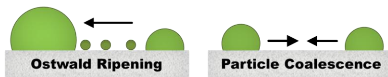
Figure 1.3. Schematics of two possible mechanisms corresponding to metal sintering
