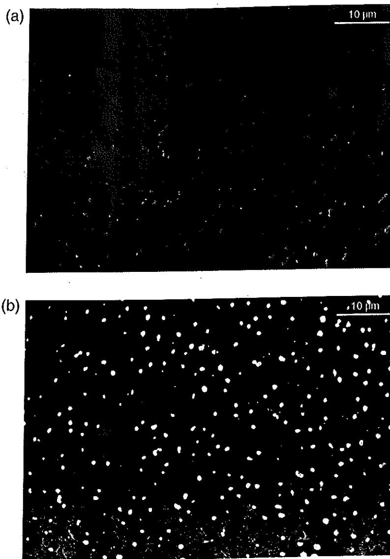
Figure 1. Epifluorescence micrographs of a K. pneumoniae biofilm on 316 stainless steel stained with (a) Rh 123 and (b) CTC (formazan) and DAPI (green), using a Leitz filter block H.
