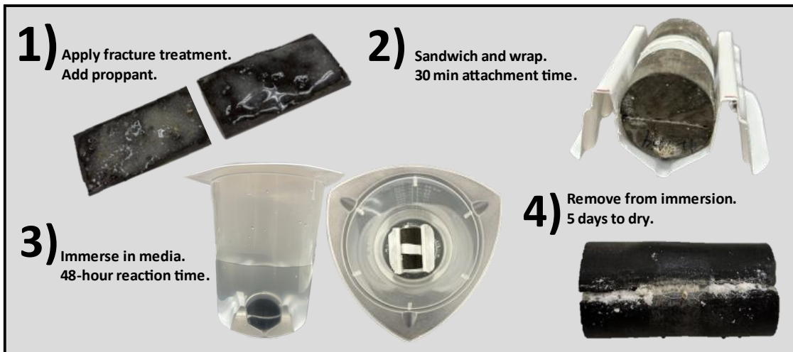
Figure 3.3. Immersion Method. 1) Apply ~3 mL fracture filler to fracture faces and sprinkle with 0.5 g proppant. 2) Sandwich cores halves together and wrap 1/2-inch Teflon tape around center of core. Let sit at the designated temperature; room temperature or 60°C; for 30 minutes. 3) Immerse into U+C media, at designated temperature, for 48 hours. 4) Remove from immersion after 48 hours and place in 40°C incubator to dry for five days. After five days, take out of incubator, remove Teflon tape, and inspect for sealing. Sealing is successful when the two core halves are attached to one another without the aid of tape.
