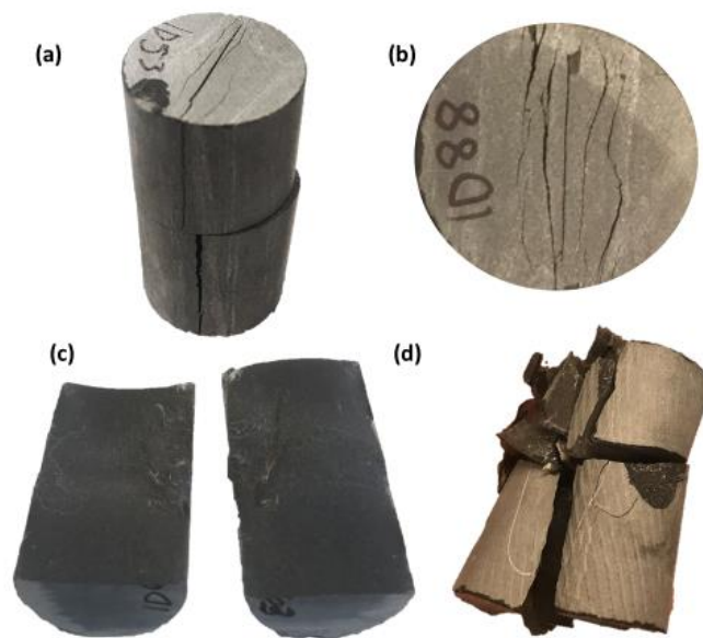
Figure 2.9. One representative core per sample group fractured in this study. (a) EF-53 tested at room temperature experienced multiple central fractures and broke in half axially. (b) The face of EF-88 tested at 60°C showcasing multiple central fractures. (c) WC-63 tested at room temperature demonstrating one “clean,” central fracture. (d) WC-68 tested at 60°C had the highest tensile strength in the study at 8.52 MPa.
