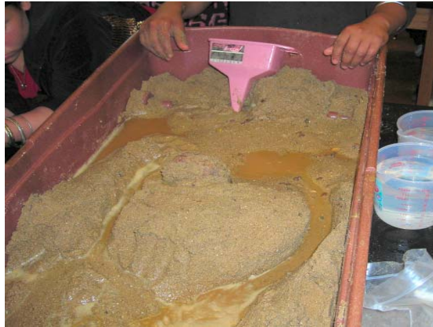
Figure 19. Students Dig a Channel (Left) to Divert Water From the Area Where They Want to Build a Dam (Right).
