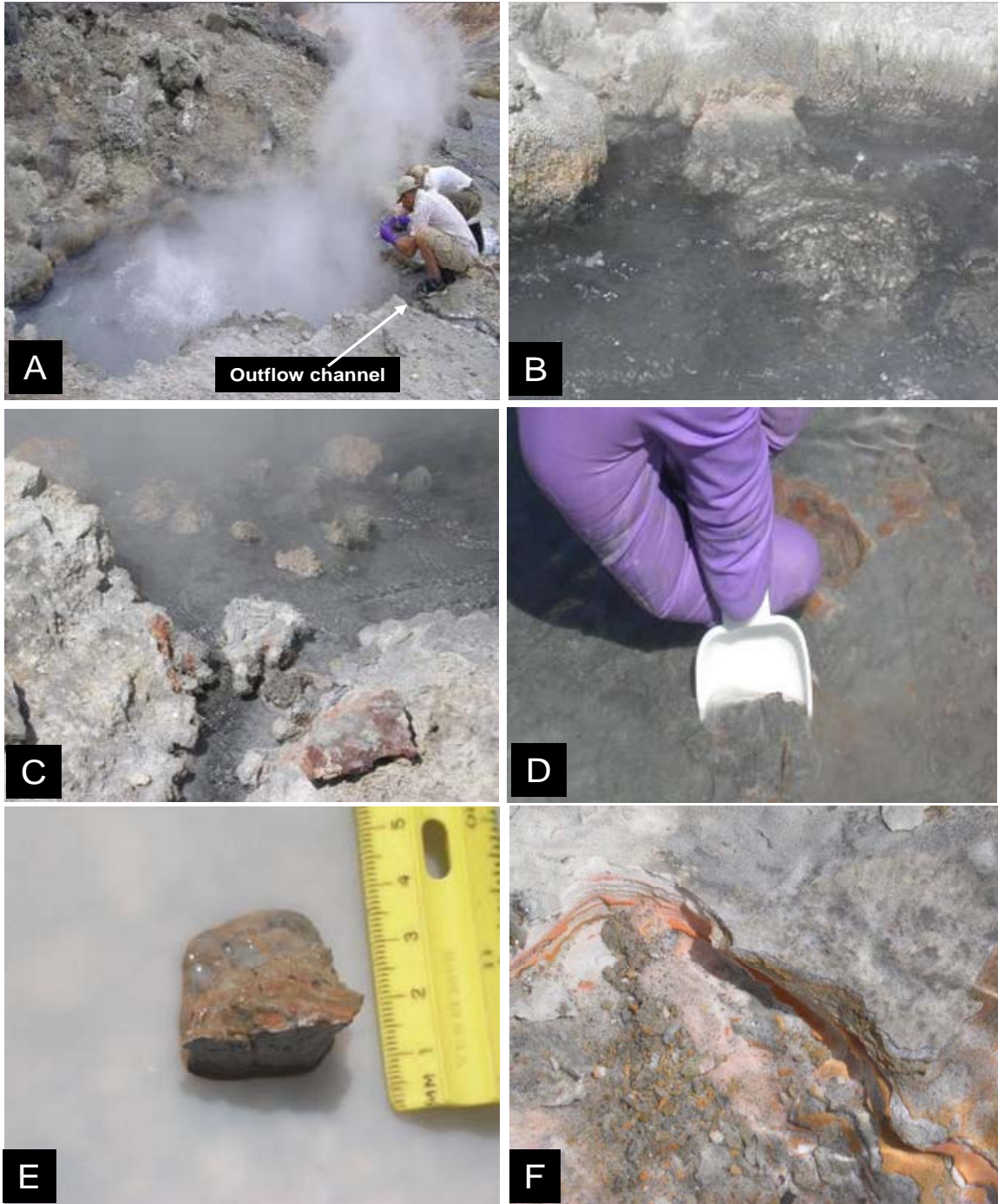
Figure 2.2. A. JC3 source pool showing the location of the outflow channel. B. Close-up of the unique metallic solid phases formed in the JC3 source pool. C. Photograph showing the outflow channel exiting the east side of the source pool. D. Sampling the source pool shelf sediments E. Core sample from shelf sediments showing stratification F. Stratified layers in outflow channel sediment. Photos were taken in August of 2004.
