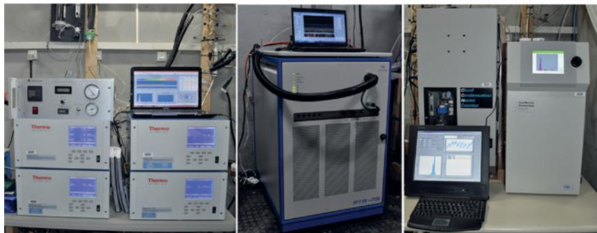
**FIG. 3. (left) Analyzers of ozone, carbon monoxide, sulfur dioxide, and nitrogen oxides were used to investigate the chemistry within and above the rain forest canopy. (middle) A PTR-MS provided concentrations of hydrocarbons. A fast mobility particle sizer recorded the physical size and concentration of aerosols. (right) A CCN counter generated concentrations of CCN based on five supersaturation levels.**
