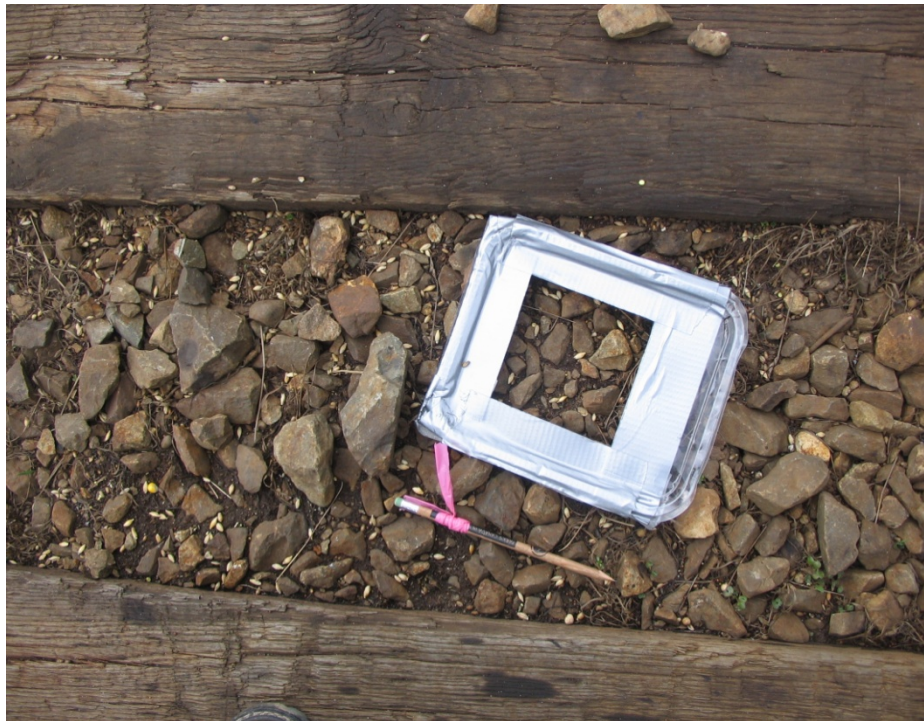
Figure 10. Grain spill sampling method used on rail bed. The grain spill sampling frame ( 10\text{cm}^2 ), used with three replicate random throws to estimate the mean density of wheat and barley seeds within a 5 m zone.
