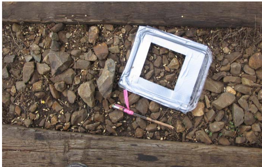
Figure 3. Grain spill sampling methods used on rail bed. a) Grain spill monitoring screen covering a 0.37\text{m}^2 area between the tracks, used to estimate the weekly weight of grain spilled at four locations. b) Spatial grain spill sampling frame ( 10\text{cm}^2 ), used to estimate the weekly weight of grain spilled at four locations. b) Spatial grain spill sampling frame ( 10\text{cm}^2 ), used with three replicate random throws to estimate the mean density of wheat and barley seeds within a 5 m zone.
