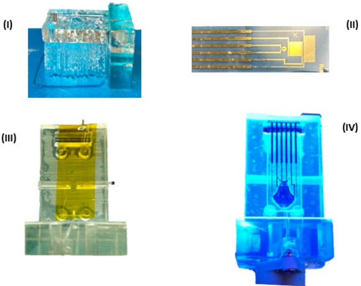
Figure 8: MSM Fabrication steps. 3-D print the MSM in the orientation shown (I). Ultrasonically clean and treat the sensor with bond-silane in preparation for packaging (II). Sand off supports and clean 3-D print in preparation for packaging (III). With a syringe and fine tip needle, draw a
