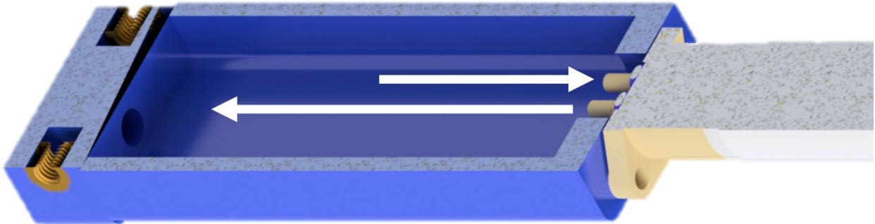
Figure 11: Cleaning Solution Module (CSM). A Lee Company micro-dispensing pump is mounted to the top of the reservoir containing 12 milliliters of 100 \mu\text{S cm}^{-1} conductivity solution.
