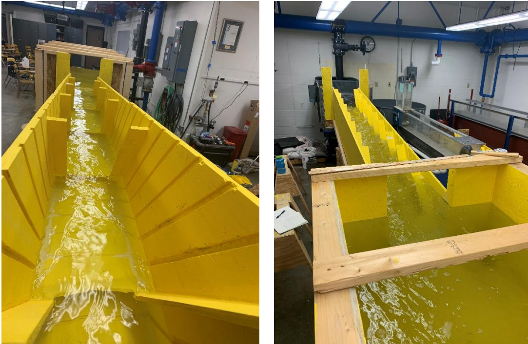
Figure 2.8: Photos of the prototype scaled Denil fishways in the MSU hydraulics laboratory set up for hydraulic testing. The left photo shows the grooves cut into the sides of each Denil to allow for baffle spacing analysis. The right photo shows Den75 full of water and provides an idea of flow conditions tested.
