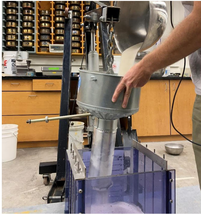
Figure 4-3. – Demonstration of pluviation process and device used in the soil compaction process for the 30-centimeter-by-30-centimeter specimen.
