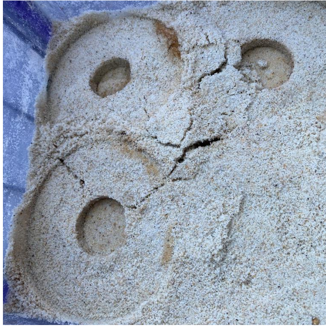
Figure B3. – Example of fissures that developed during the CBR testing of the 30-centimeter-by-30-centimeter specimen, potentially contributing to the lower CBR values returned in some areas.
