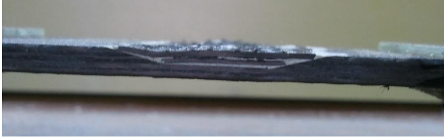
Figure 32: Edge View of Completed PMMA 50% Repair Specimen with 5 Degree Scarf Angle
