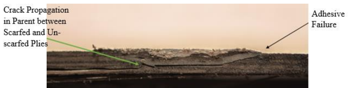
Figure 48: Failure of Un-scarfed Plies Leading to Ultimate Failure in a 15 Degree, 50% Repair Specimen
