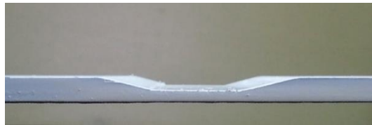
Figure 25: Edge View Milled Repair Specimen, 15 Degree Scarf Angle, 50% Through Thickness Repair (Painted white for ARAMIS DIC imaging purposes)
