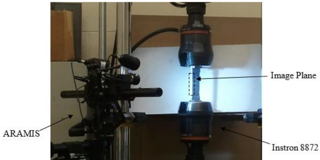
Figure 23: Static Tension Test Set Up for Joint Specimens
