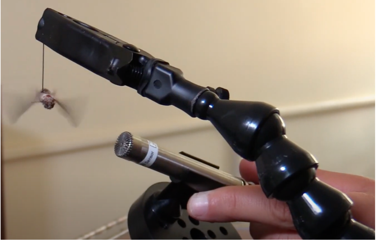
Figure 20: Setup for the wingbeat frequency measurements using a piezoelectric microphone. An army cutworm moth, suspended on a pin, was held by a vice (upper left). A piezoelectric microphone was placed underneath the moth to measure wingbeat frequency.
