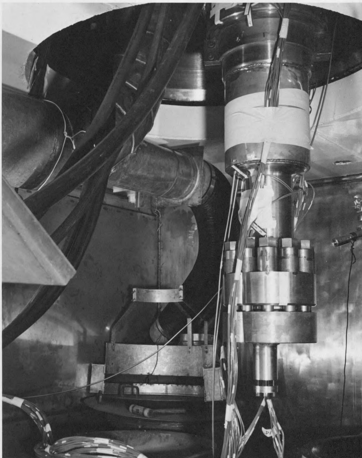
Fig. 8 - Lower end of completed vessel assembly in test cell.
