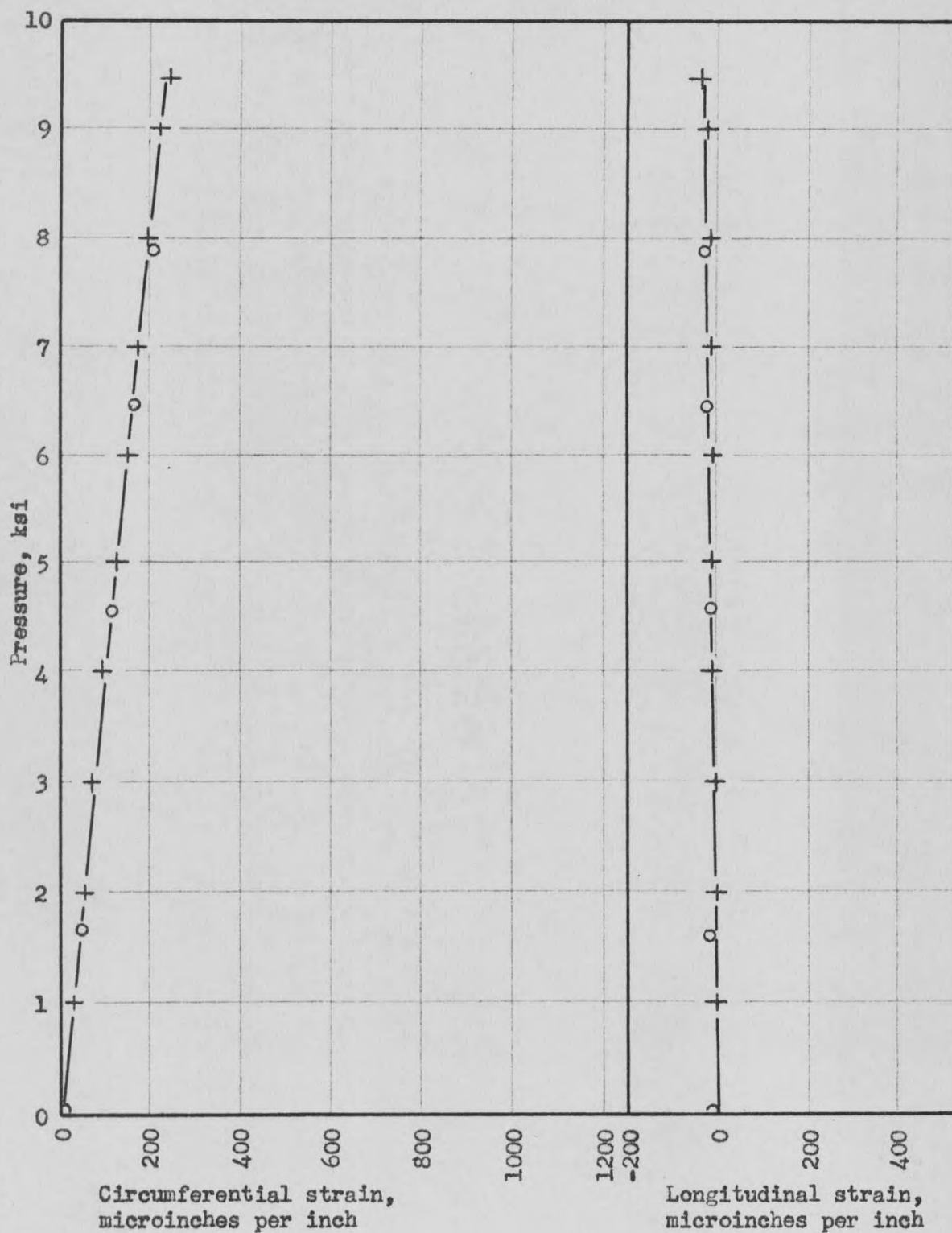
Fig. 41 - Pressure vs strain at section J, test #3.
