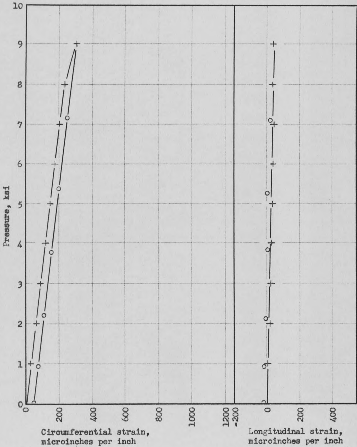
Fig. 37 - Pressure vs strain at section I, test #2.
