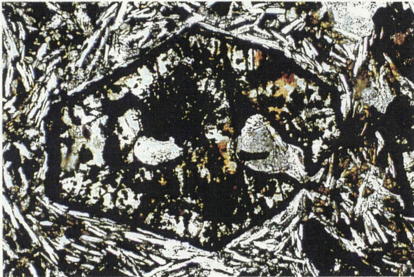
Figure 5. Photomicrograph of Sample 81 (PPL, 85x). Olivine phenocryst altered to fine-grained opaques.
