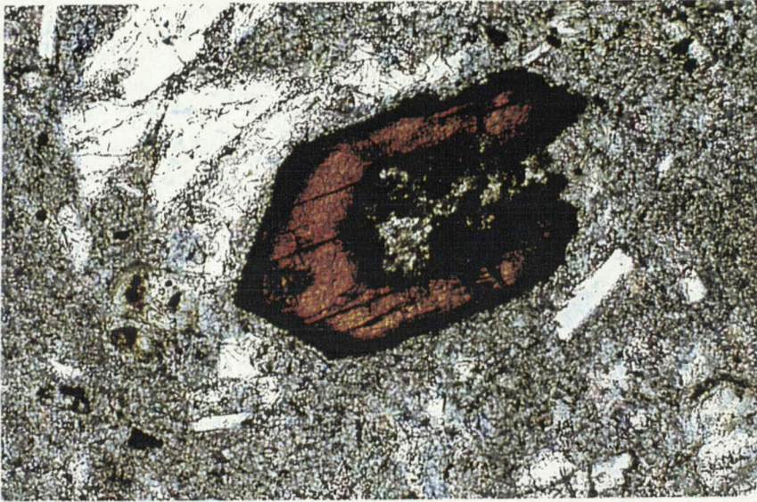
Figure 11. Photomicrograph of Sample SM2 (PPL, 85x). Biotite with oxide reaction rim due to dehydration.
