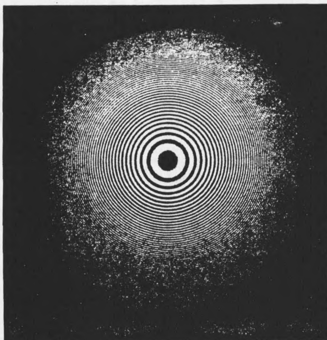
Figure 19. A typical transmitted interference pattern of a Fabry-Perot etalon.
