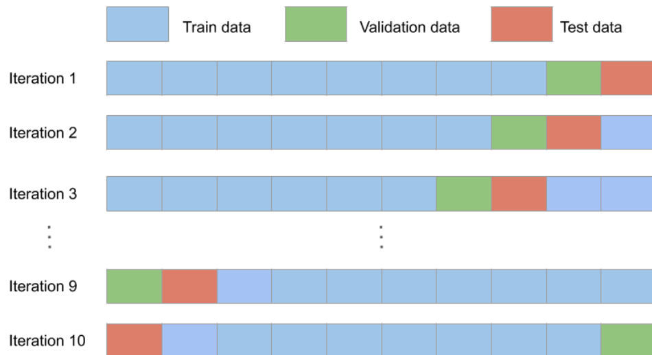
Figure 3.6: Representation of the stratified train, validation and test setup for SVMs model
