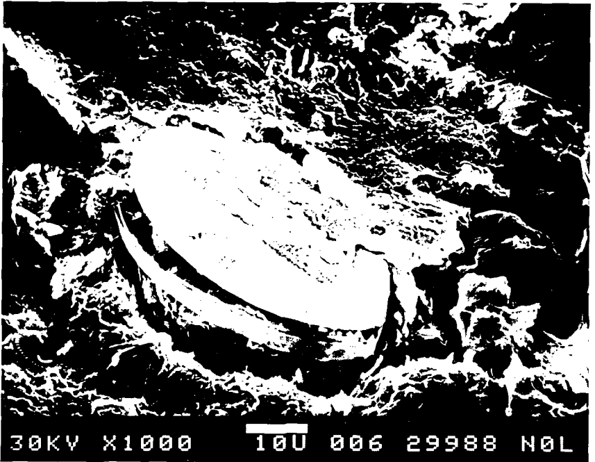
Fig. 8 SEM micrographs of biofilm from Gulf of Mexico water formed on S30400 during continuous illumination.
