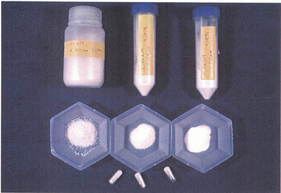
Fig. 4.1. Photo of Pantoea agglomerans strain Eh 239 formulated in the oil/starch/sugar encapsulation method (USDA) developed by Quimby et al., 1996. Bacterial formulations were sieved after air drying in granule sizes of 250-750 \mu\text{m} , 150-249 \mu\text{m} , and <math>< 150 \mu\text{m}</math> and stored as wettable powders in plastic containers or gelatin capsules.
