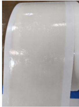
Figure 2.10: Resin film of uniform thickness to be applied to the 10 tow wide stretch broken ribbon
