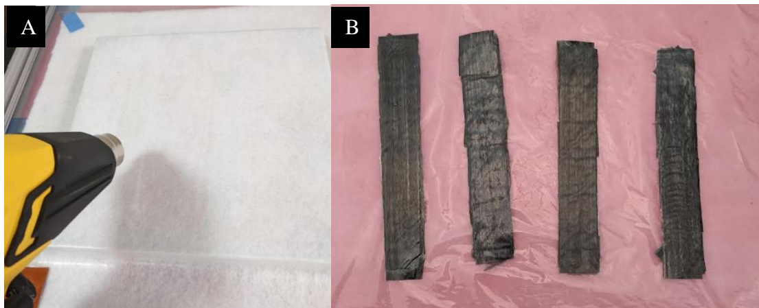
Figure 4.15: (A) Heat gun/vacuum consolidation (B) Prepreg layup [0/+45/-45/90]_s
