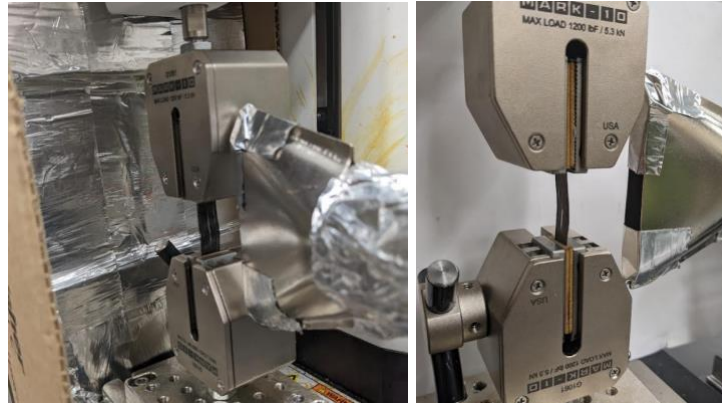
Figure 3.3: Heat gun equipped with different nozzles used for elevated temperature testing
