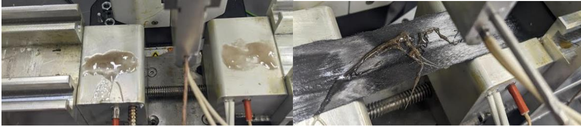
Figure 5.11: Extra resin placed between the tool and the ply
