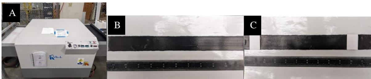
Figure 5.2: (A) Prepreg fusing compaction machine (B) Prepreg cut into sample length (C) Prepreg tabbed and ready for testing
