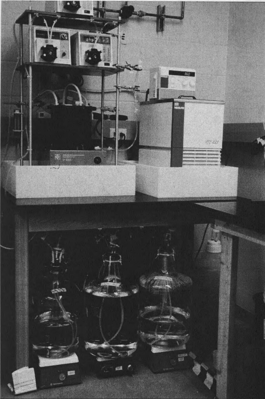
Figure 4. Photo of biofilm annular reactor laboratory system
