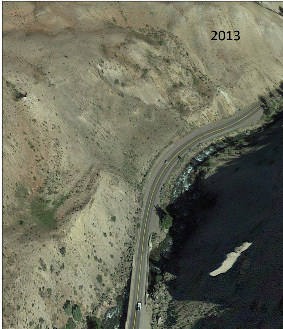
Figure 11B. Same area of photo 10B showing a smoothed surface where the reactivation occurred in landslide five that was modified by the park service. This photo was taken in 2013 and was downloaded from Google Earth.
