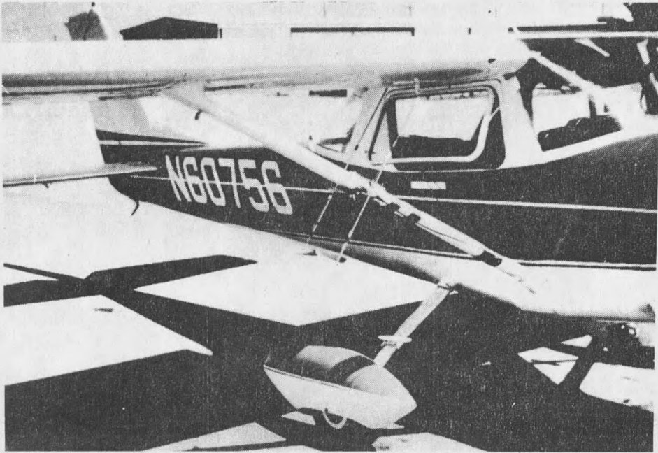
Figure 13. Telemetry receiving antenna position on high wing aircraft. Antenna was mounted for reception of signal from front of aircraft.
