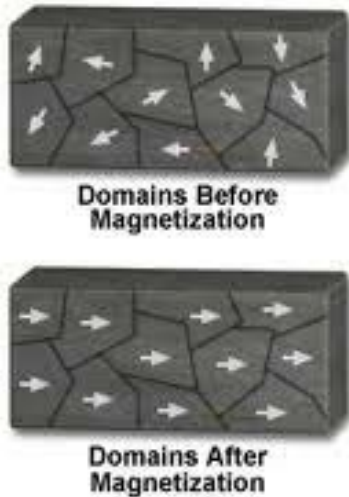
Figure 13. Domains of a Material Before and After Magnetization.
