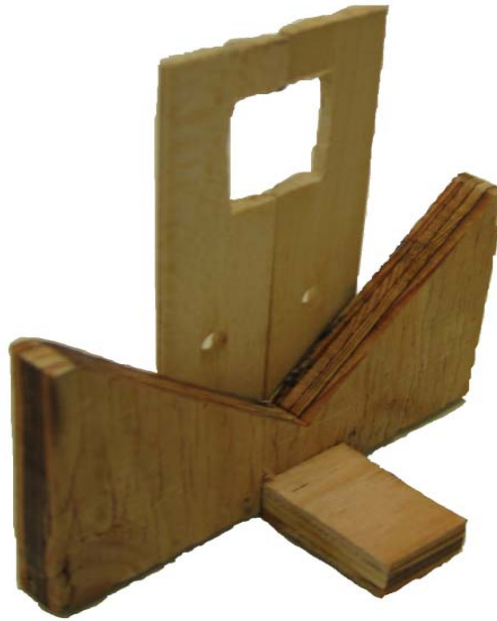
Figure 16: Jig created to position membranes in the center of the rheometer base plate.
