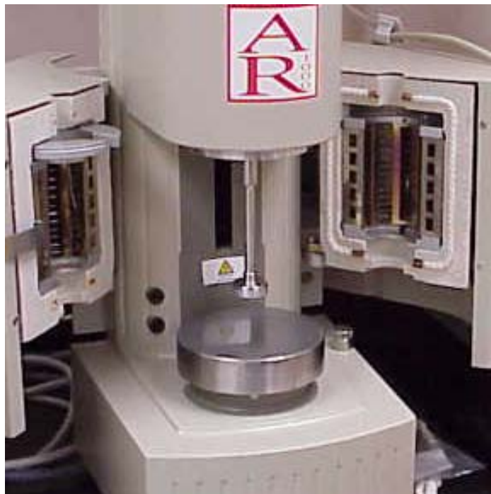
Figure 14: TA Instruments AR1000 rheometer used to perform creep tests.
