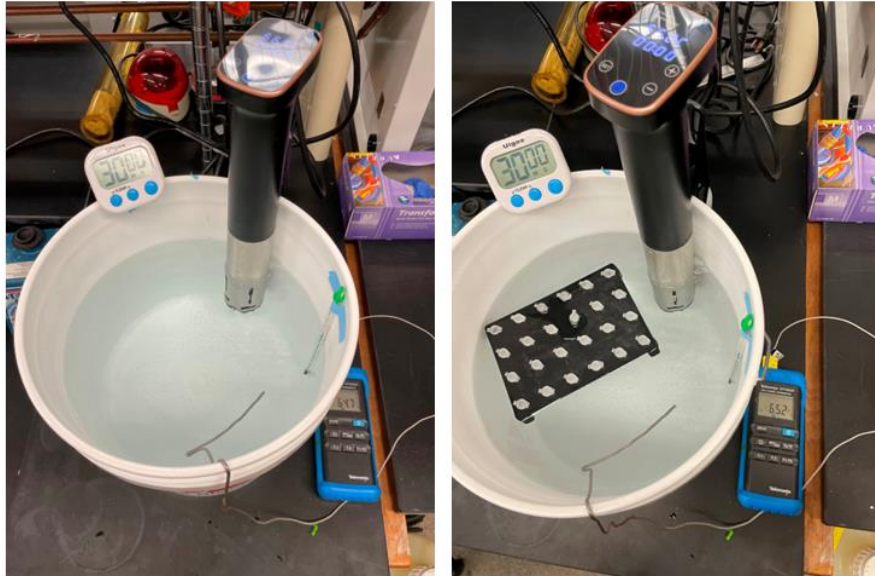
Figure 8.7. Sous vide incubation setup. (Left) Example of sous vide incubation set up including circulating heater, thermometer, thermocouple, and timer. Water temperature is checked independently by both analog thermometer and thermocouple to hold nominal temperature of 65C. (Right) Image of microcentrifuge tubes in a floating 3D printed rack.
