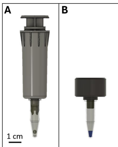
Figure 6.1. Render of point-of-care (POC) devices for RT-LAMP based assays. (A) Render of POC device designed for patient activation, featuring a plunger mechanism that actuates an integrated liquid-filled blister. This design is handheld and ergonomically optimized for thumb activation, similar to the action of clicking a pen (see Chapter 7). (B) Render of a minimized device body, providing proof-of-concept device for testing assay workflow. This design is optimized for packing efficiency, material use, and automated handling but is not a fully functional POC prototype (see Chapter 8). Scale bar represents 1 cm.
