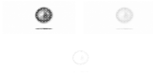
Figure 5.13 Images with OD 0, OD 1.6 and OD 4 in direct detection
