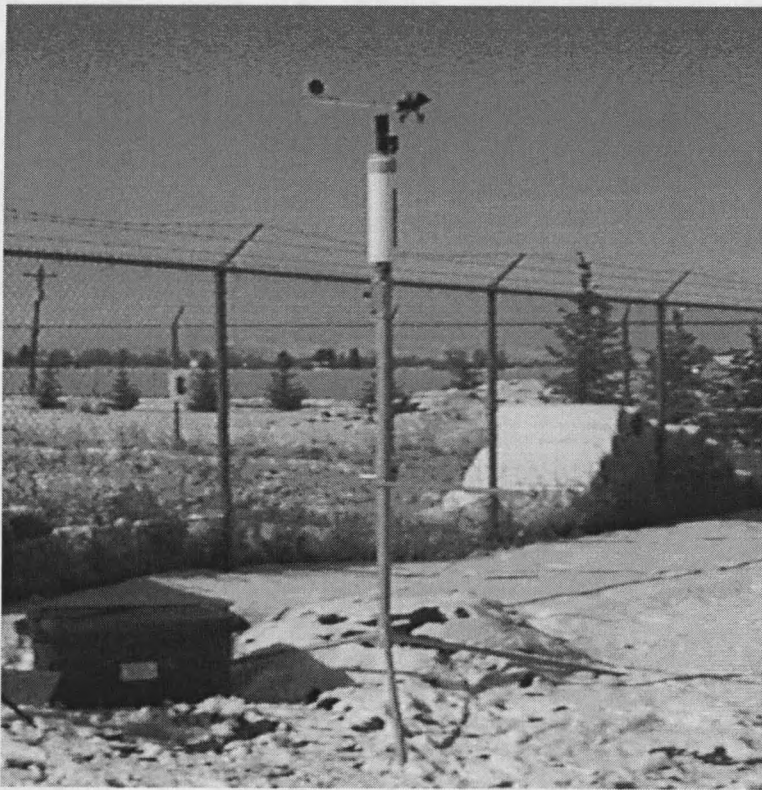
Figure 17. Picture of the WEATHERPAK-400 and the Li-Cor pyranometer at the test site. [The Li-Cor pyranometer is mounted on the horizontal bar].
