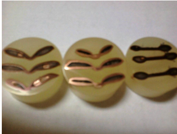
Figure 24: Image of crimped samples mounted in epoxy and polished
