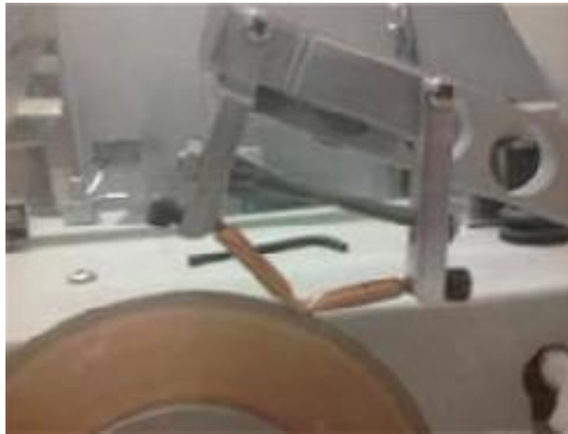
Figure 21: Image of holding fixture clamped onto tube and Buehler Isomet 1000 saw
