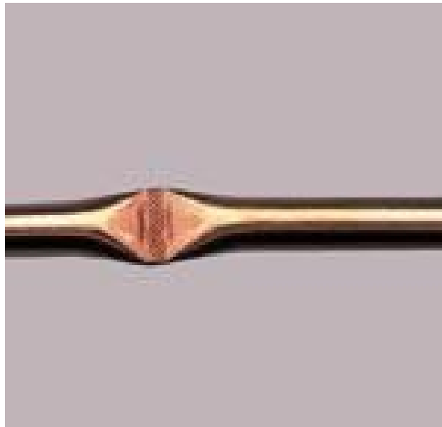
Figure 4: Image of a tube crimped by the “Tube Terminator” [3]
