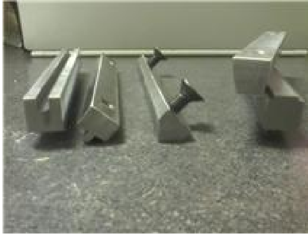
Figure 11: Image of hammer and anvil pairs which mimic the shape of sponsor's dies
