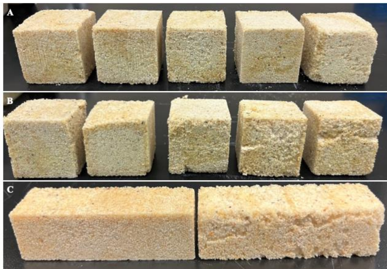
Figure 9. Biocemented specimens after 3 injections. A) 50 x 50 mm cubes prepared using APMDES-treated sand. B) 50 x 50 mm cubes prepared from non-treated sand. C) Prisms (25 x 25 x 90 mm) prepared from APMDES-treated sand (left) and non-treated sand (right).
