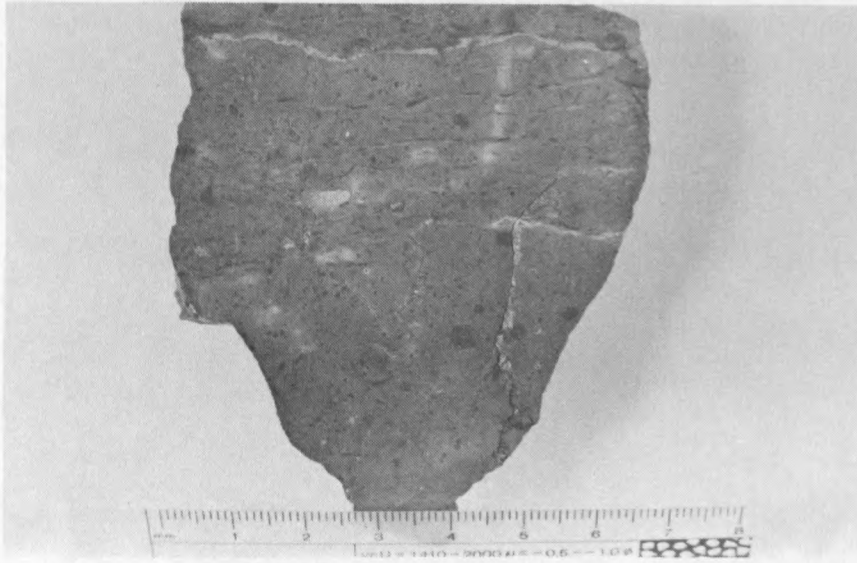
Figure 11. Photograph of a slab of the calcareous layer showing rounded clasts of host mudstones and veins of sparry calcite.
