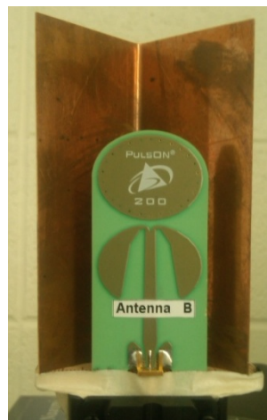
Figure 43. A 90^\circ corner reflector of copper is added to the Pulse ON 200 antenna.
