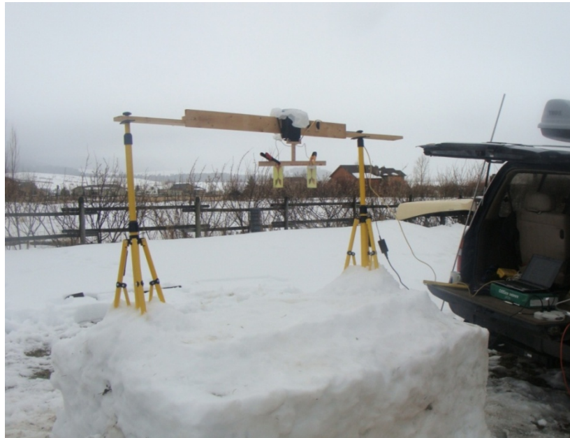
Figure 91. Experiment setup for measuring snow depth using the Pulse ON 220 radar system and the Vivaldi antennas.
