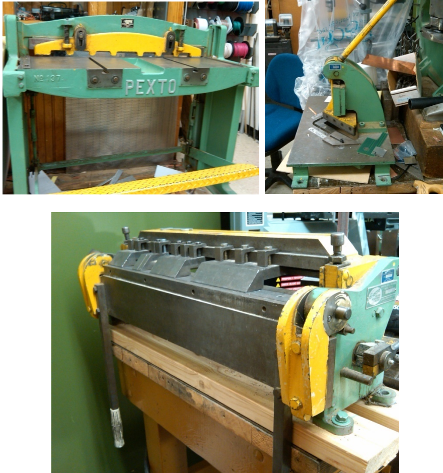
Figure 19. Stomp shear (top left), corner notch (top right), finger break (bottom) machines at the stock room in the ECE department.
