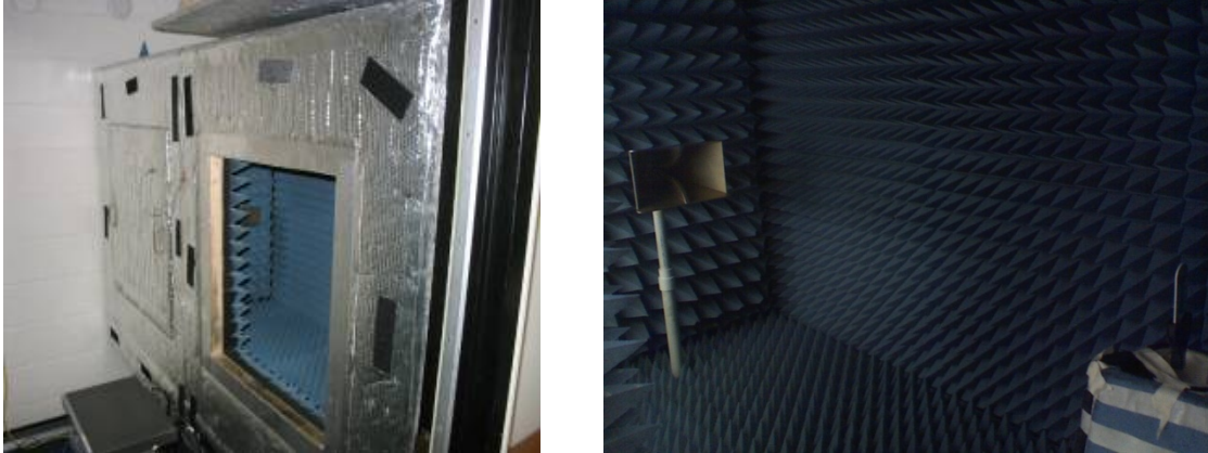
Figure 23. The anechoic chamber (left) used for testing antennas eliminating secondary reflections, and the interior of the anechoic chamber (right) containing the horn antenna on the left and the tested antenna on the right
