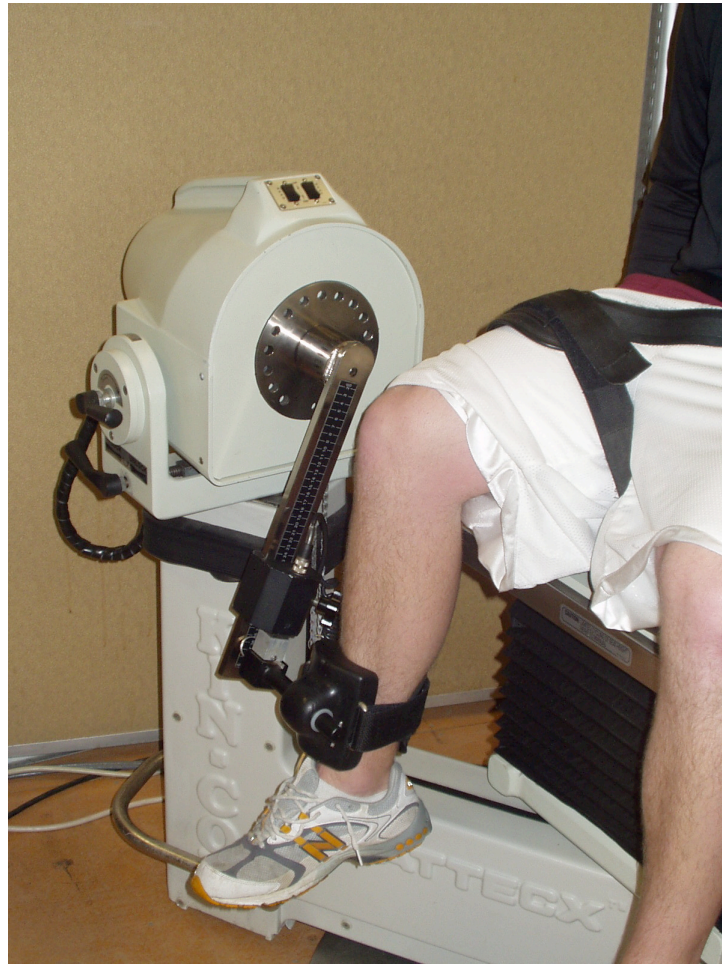
Figure 3.5: Setup of leg to lever arm and force transducer of the KIN-COM dynamometer.
