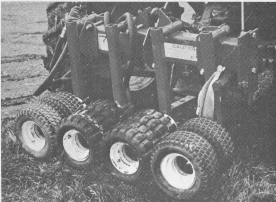
Figure 5. The tractor mounted, hydraulically driven Bourquin Weed Puller (Bourquin Design and Mfg., Colby, Kansas) design for pulling weeds from row crops.
