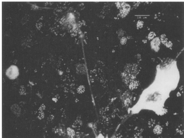
Figure 1 Scanning confocal laser micrograph of a biofilm that developed on a glass surface in a modified Robbins device irrigated with river water. The biofilm was prepared for microscopy by fixation with glutaraldehyde and treatment with the protein-binding stain, rhodamine isothiocyanate. This image is a projection of twenty optical sections through the biofilm, obtained at 1- \mu m intervals. The biofilms that developed in this system were complex communities consisting of various bacterial morphotypes, as well as algae (diatoms) and protozoa
