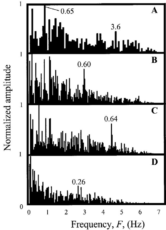
**Figure 6.** Power spectra of oscillatory streamer motion generated from fast Fourier transform analysis of the time trace data at various  $u_{(ave)}$ ; (A) 1.2, (B) 4.7, (C) 6.9, and (D) 9.5 cm/s. Isolated peaks were identified by eye and are shown with their associated frequency to flow velocity ratio ( $\text{cm}^{-1}$ ).
