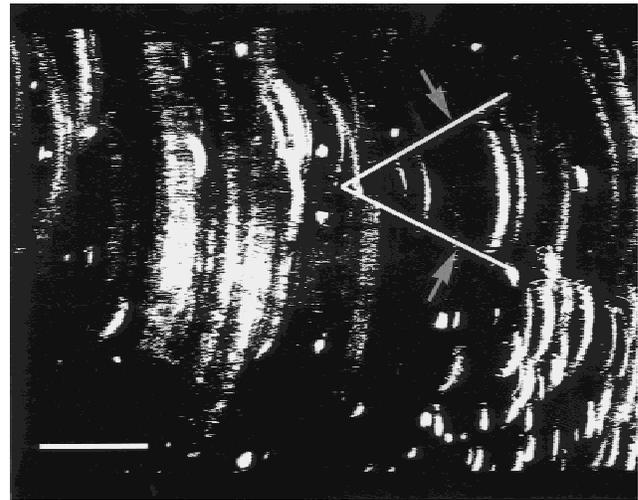
**Figure 3.** Time exposed image of fluorescent beads attached to biofilm streamers show the oscillating streamers formed arc shaped paths. The two white lines (shown by arrows) indicate the maximum displacement envelope (twice the maximum amplitude) of one of the streamers. Flow direction was from left to right. Scale bar = 500  $\mu\text{m}$ .
