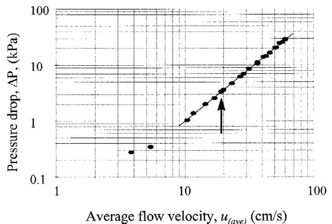
**Figure 1.** Relationship between pressure drop ( $\Delta P$ ) and average flow velocity ( $u_{(ave)}$ ) for a clean flow cell. The closed circles are measured data. The solid line is the regression line calculated from data above 10 cm/s and indicates the turbulent region of the curve. The gradient of the regression line (1.84) is the velocity exponent,  $m$  in Eq. (2). The biofilm was grown at a flow velocity of 18 cm/s (shown by arrow).
