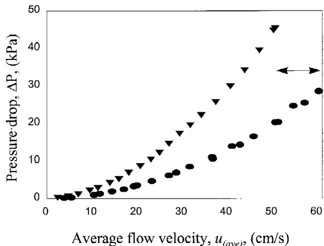
**Figure 4.** Relationship between pressure drop and flow velocity for a clean flow cell (circles, same data shown in Fig. 1) and for a flow cell colonized with biofilm (triangles). Biofilm colonization in the flow system resulted in a 16% decrease of achievable flow rate (indicated by the arrow).
