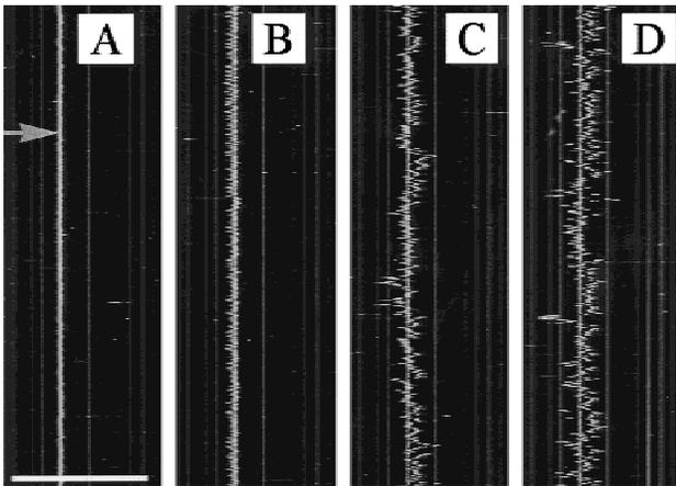
**Figure 5.** Time trace of streamer displacement (shown by arrow) at various  $u_{(ave)}$ ; (A) 4.7, (B) 9.5, (C) 11.3, and (D) 16 cm/s. The time traces were made by repeatedly scanning the line shown in Figure 2A that intersected the streamer indicated in the same figure. The X axis represents distance and the Y axis time. The negative of the original image is shown for clarity. Scale bar = 500  $\mu\text{m}$ .
