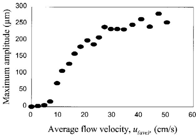
**Figure 7.** The maximum amplitude of the biofilm streamer shown in Figure 2A increased with  $u_{(ave)}$  in a sigmoidal shaped curve.
